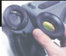
Interchangeable lens options enable adjusting to an ideal field of view
